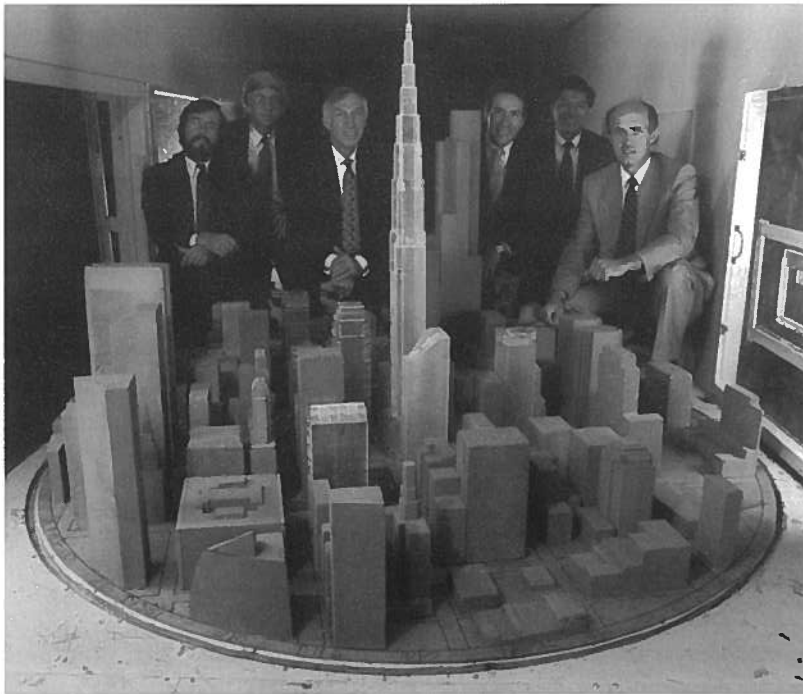
1:400 pressure model of Miglin-Beitler Tower in Rowan Williams Davies & Irwin's Boundary Layer Wind Tunnel in Guelph, Ontario. Visitors are: (from left) Gregg Jones of Cesar Pelli & Associates, Charles Thornton of Thornton-Tomasetti Structural Engineers, Lee Miglin and Paul Beitler, and Ray Chin of Miglin-Beitler and Dr. Peter Irwin, RWDI's Principal-in-Charge.
