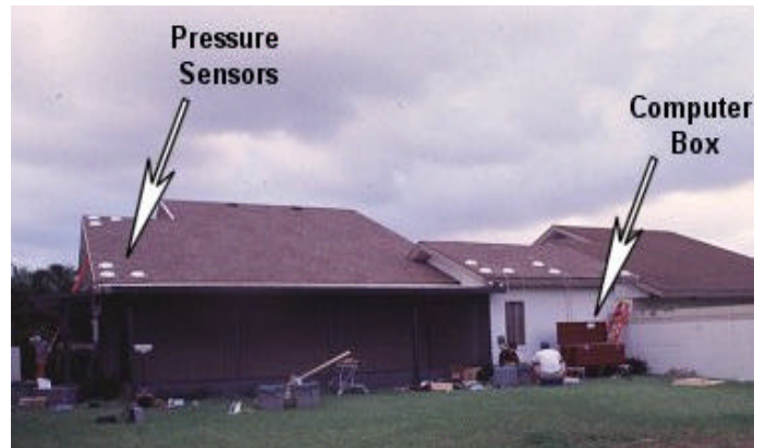
Fig. 3. Jupiter, FL House Being Outfitted with Sensors to Measure Hurricane Floyd in 1999
