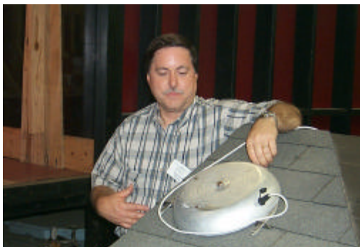
Tim Reinhold Describes Pressure Transducer (used in field studies) During Tour of Wind Engineering Laboratory at Clemson University
